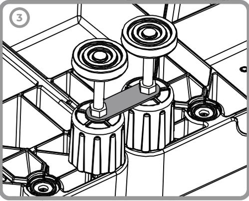
(3) IF USING WITH THE EXTENDING FOOT FEATURE ENSURE THE LINK BAR IS BETWEEN THE BOTTOM OF THE EXTENDING FOOT AND THE LOCKING NUT.
