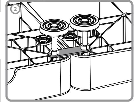
(2) SCREW FEET THROUGH THE LINKING BAR AND TIGHTEN UP SECURELY SO THE THE LOCKING NUT IS FIRMLY AGAINST THE LINKING BAR.
