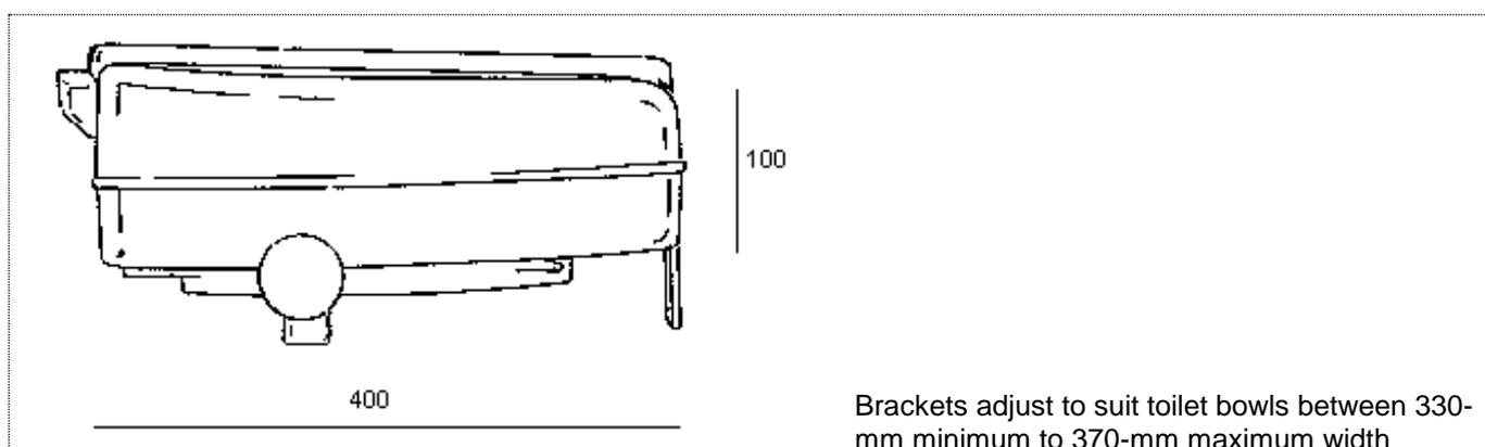
Brackets adjust to suit toilet bowls between 330-mm minimum to 370-mm maximum width
